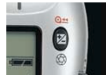
Aperture/Exposure compensation button Press this button while rotating the Command Dial to select aperture in Manual exposure mode.
